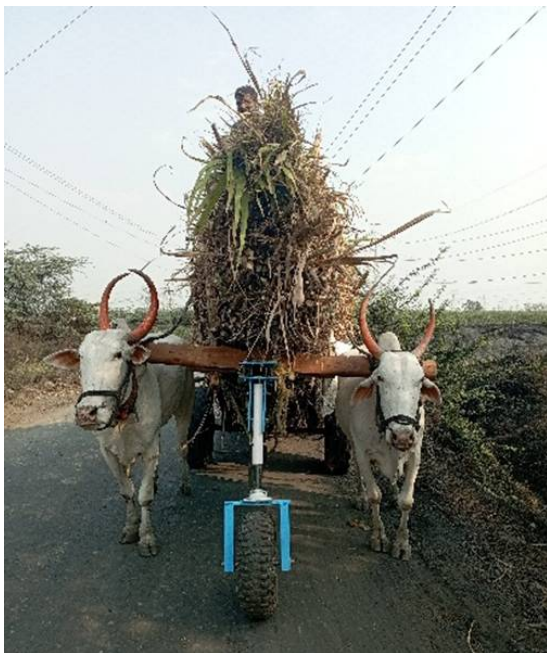
Third Rolling Support Mechanism for Bullock Cart
